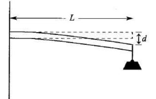
A weight is hung at the end of a beam of length L. This causes the end of the beam to drop a distance d. d is directly proportional to the cube of L. d = 20 when L = 150.
