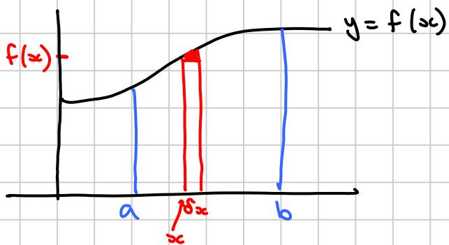
We can think of an area under a curve as being made up of strips, each of which is  $\delta x$  wide. Each strip is approximately a rectangle  $f(x)$  high ( $f(x)$  is different for each rectangle).
