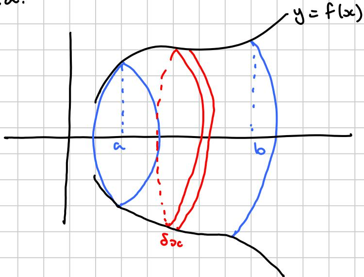
We can visualise this solid as made up of discs which are approximately cylinders with " $h = \delta x$ " and " $r = f(x)$ ".
